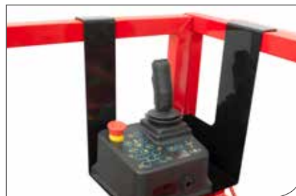
Ergonomic and removable control panel
