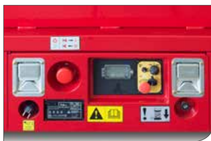
Ground control panel
