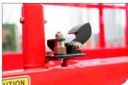
Pedal locking for platform extension
